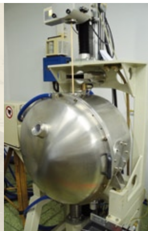
Device for growing single crystals with the Czochralski method, photo by A. Duda-Nowicka
